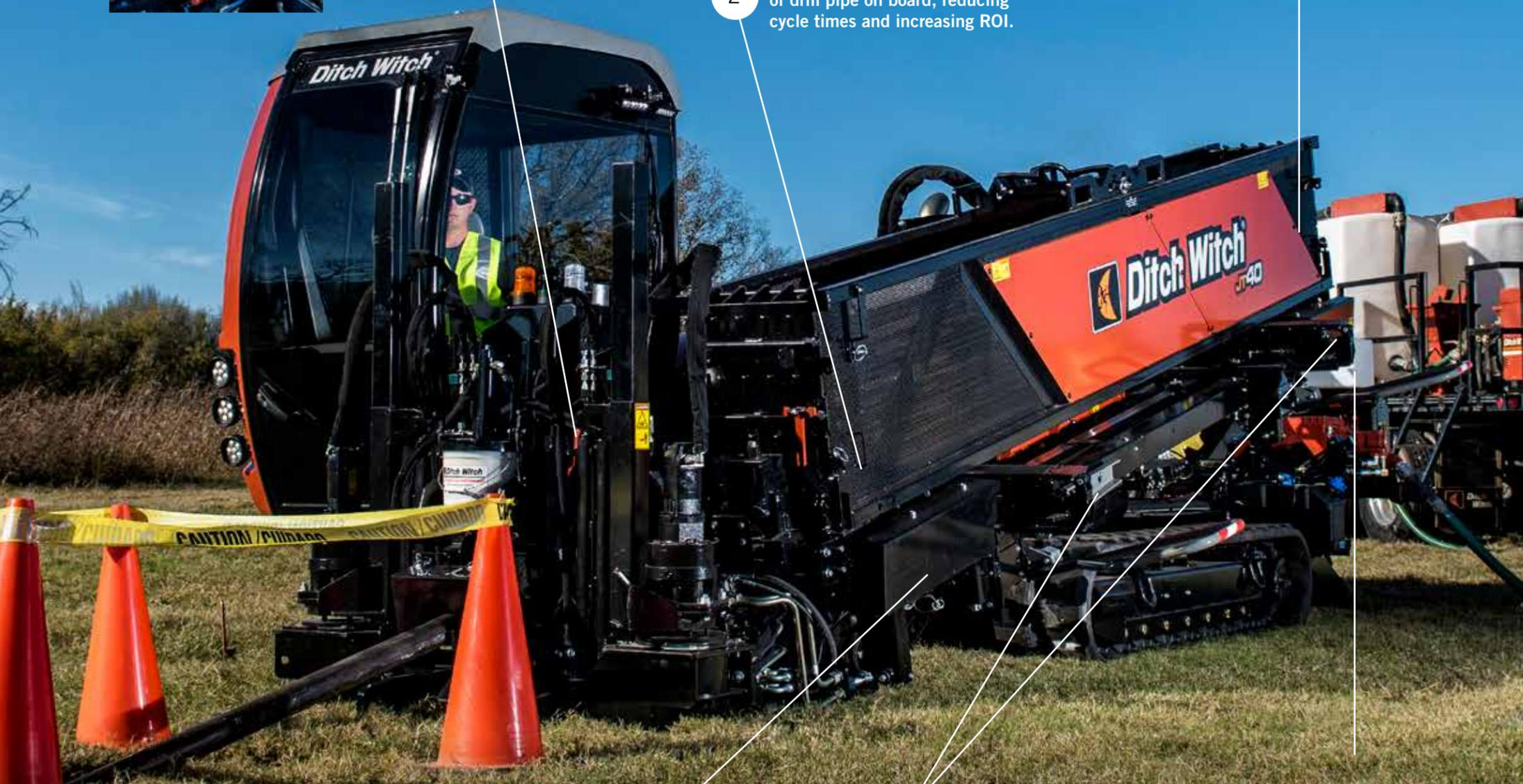
6 The new patent-pending slide cartridge allows operators to effectively complete a job, without stopping for increased uptime.
